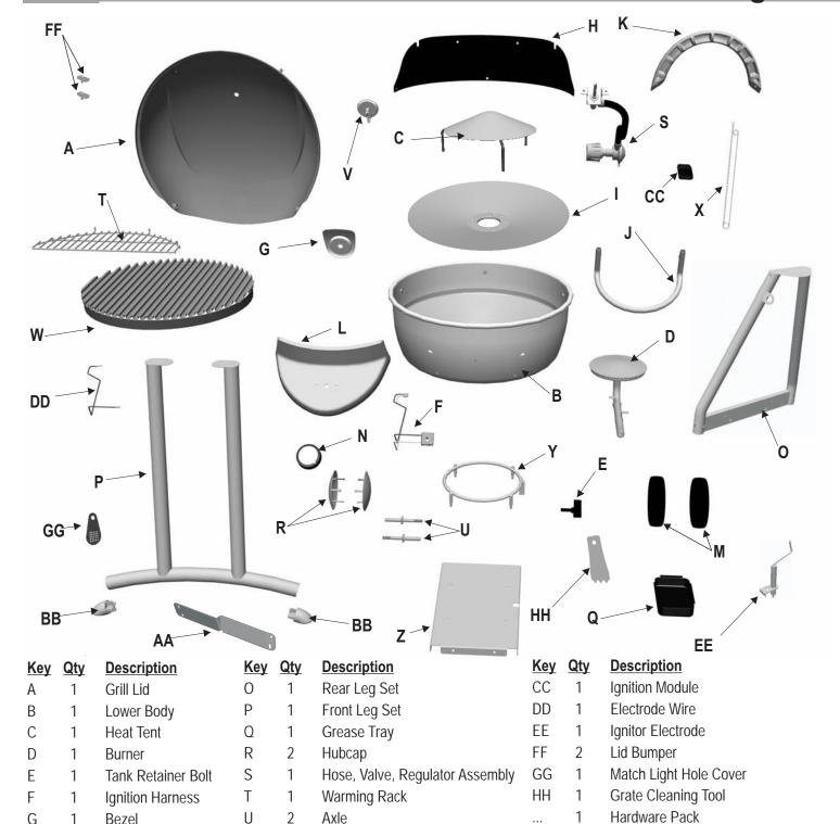
1 Control Knob BB 2 Leg Cap ... 1 Product Guide, French, Optional NOTE: Some grill parts shown in the assembly steps may differ slightly in appearance from those on your particular model. However, the method of assembly remains the same.
